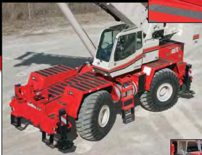
Fast & efficient hydraulic counterweight removal enhances roadability
