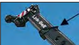
A-max extends only the inner-mid section of the boom for substantially increased capacities for in-close, maximum capacity lifts.
