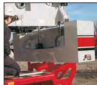
Fast & efficient hydraulic counterweight removal enhances roadability
