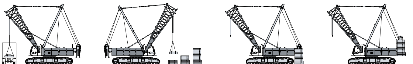
Unloading and assembly of rear counterweight
