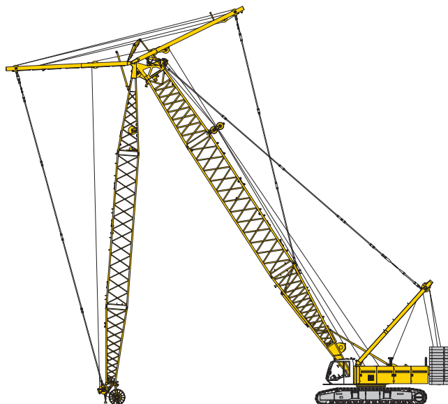
Erecting of main boom and luffing jib
