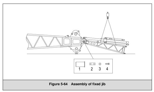
c) According to actual condition, choose and assemble several 6m fixed jib intermediate sections (G33). All fixed jib intermediate sections are connected with double tapered pins (5), secured the pins on both sides with retaining springs (6) as follows:
