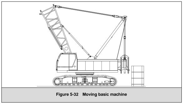
b) Travel basic machine backwards until the counterweight lifting cylinder is positioned above the mounting hole of counterweight base plate. Connect counterweight anchoring rods. See the figure 5-33.
