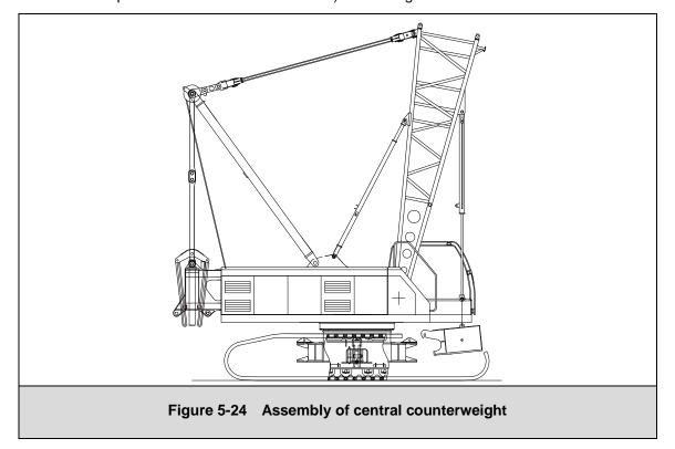
When central counterweight is aligned with the undercarriage central section, attach the hooks at the upper side of central counterweight to the attachment points on the undercarriage central section. See the figure 5-25.
