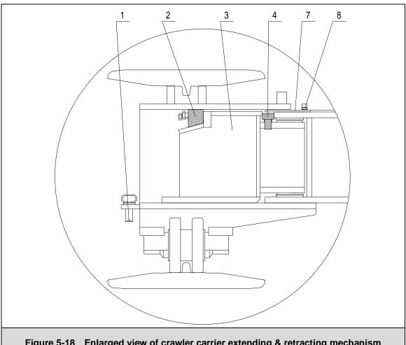
Figure 5-18 Enlarged view of crawler carrier extending & retracting mechanism
