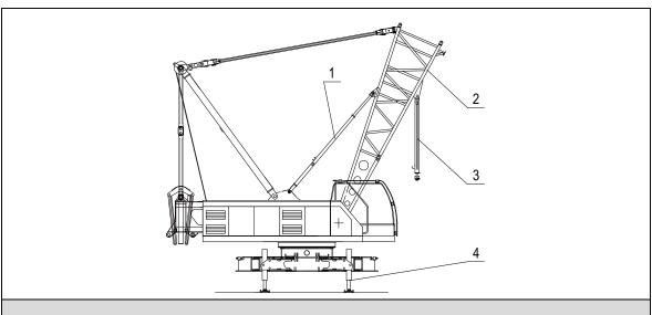
Figure 5-8 Preparation for crawler carrier self-assembly
