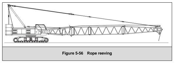
Place the load hook directly under main boom head, and then reeve the hoisting rope between hook block and rope pulley on main boom head in accordance with the rope reeving plan (for the details, please refer to section 4.6 "rope reeving" in Chapter 4), finally secure the rope end point with rope lock and rope thimble, referring to the figure 5-57.
