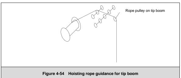
When rope reeving is 2 and the tip boom is fitted on the main boom head, the rope must be guided over the deflection pulley on the middle position of main boom head, and reeved in according to the figure 4-56.
