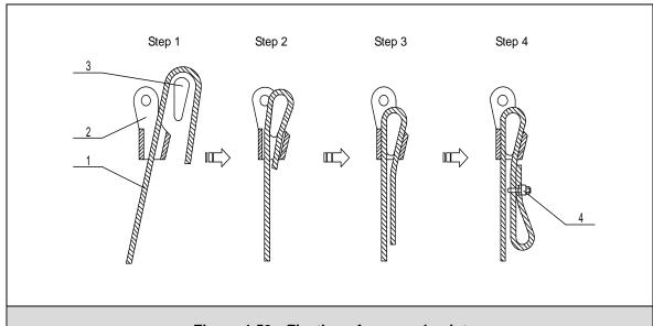
Figure 4-59 Fixation of rope end point
