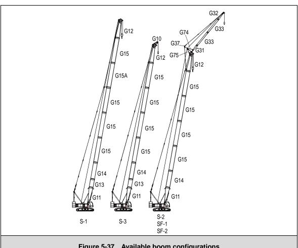
Figure 5-37 Available boom configurations
