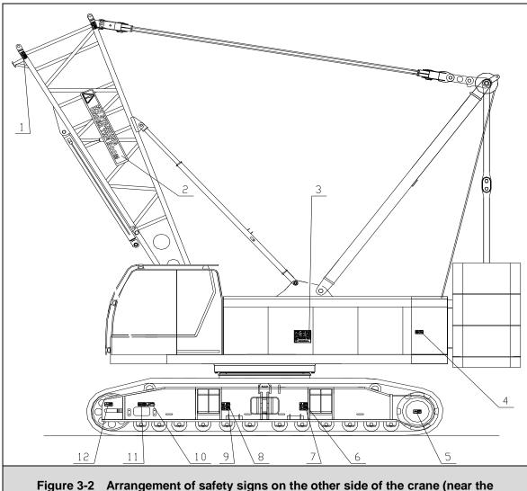
Figure 3-2 Arrangement of safety signs on the other side of the crane (near the operator's cab)
