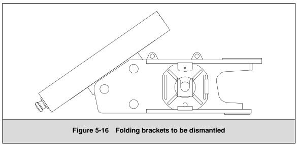
Dismantle folding brackets by use of mounting cylinder or other device, and then connect b) the horizontal anchoring rods.
