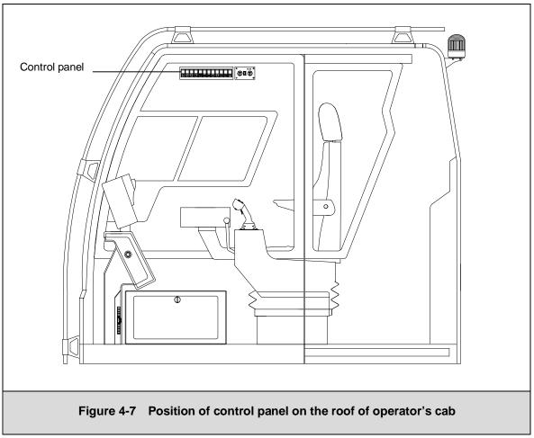
Refer to figure 4-7 for the position of control panel on the roof of operator's cab and refer to figure 4-8 for details.
