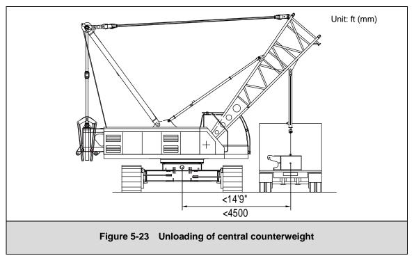
b) Raise main boom pivot section to make central counterweight move backwards, and then adjust the height of central counterweight via mounting cylinder. (Note: The angle of main boom pivot section can not exceed 84°.) See the figure 5-24.
