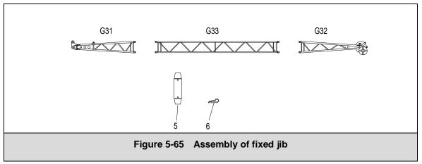
The components used to assemble fixed jib are shown in the figure 5-17.
