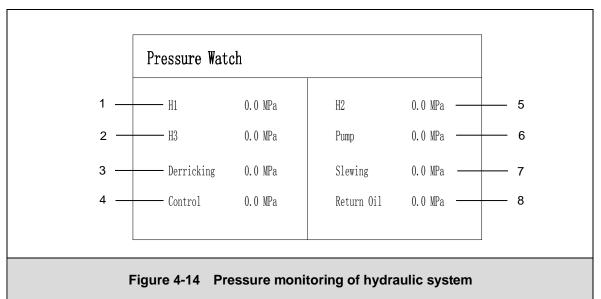
The pressure monitoring of hydraulic system will be described in details in the table 4-12.
