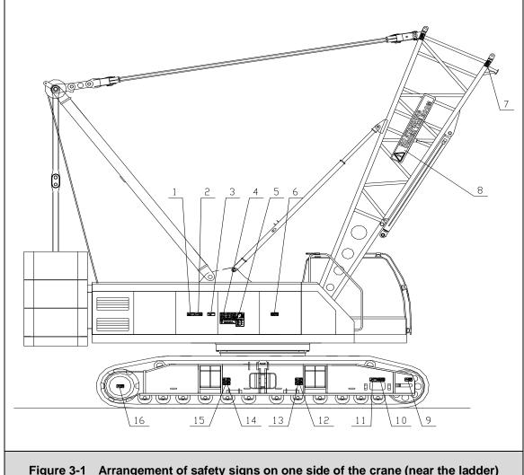
Figure 3-1 Arrangement of safety signs on one side of the crane (near the ladder)
