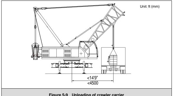
Figure 5-9 Unloading of crawler carrier
