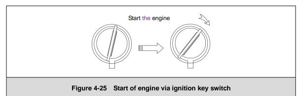
After the engine is started, check if the following items of engine are normal. See the figure 4-26.
