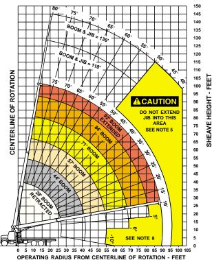
Area of Operation DO NOT OPERATE IN THIS AREA WITHOUT FRONT DEPLOYED
