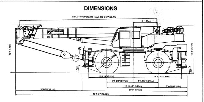
Note: Dimension is with boom angle at -1.5 degree.
