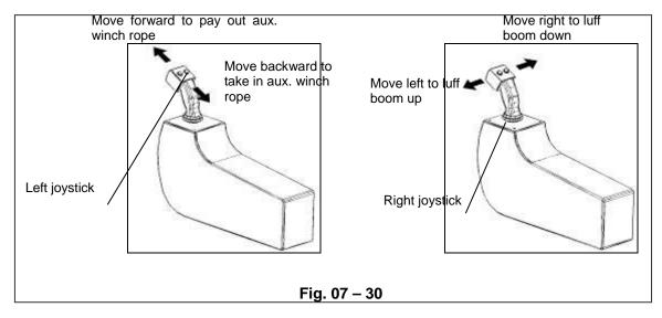
Move left and right joysticks at a time to initiate required crane movements.
