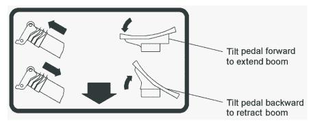
Figure 06 – 8 Boom Extend / Retract Pedal
