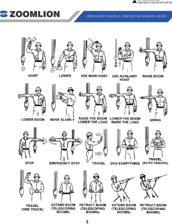
Figure 04 – 4 Hand Signals for Crane Operation
