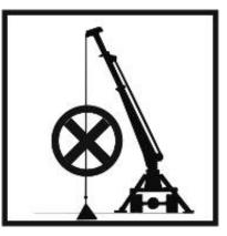
(9) Do not extend / retract the boom with a suspended load.
