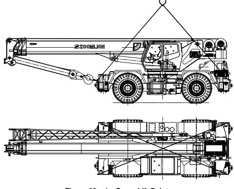
Figure 08 – 1 Crane Lift Points
