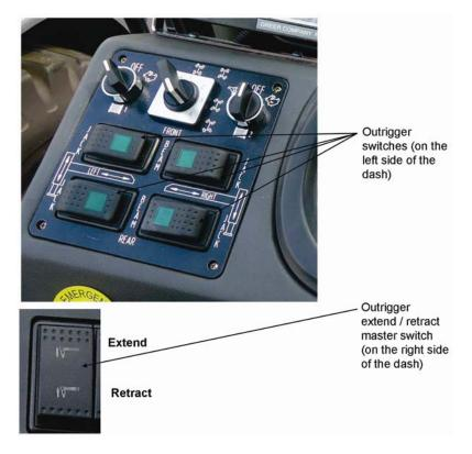
Figure 07 – 4 Outrigger Switches
