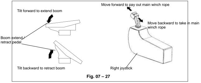
Move the right joystick and tilt the boom extend / retract pedal at a time to initiate required crane movements.
