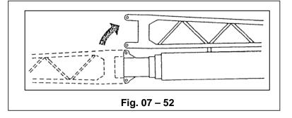
(2) Remove and store the auxiliary hook according to the conductor's hand signals.
