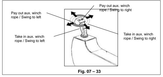
Move the left joystick between any two adjacent arrows to initiate required crane movements.
