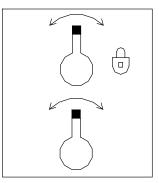
Fig. 07 – 26 SWING LOCKOUT SWITCH
