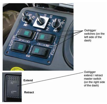
Figure 07 – 4 Outrigger Switches
