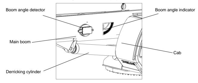
Figure 07 – 20 Boom Angle Indicator / Detector
