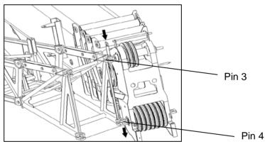
Figure 07 – 38 Pins (3) and (4) Installation
