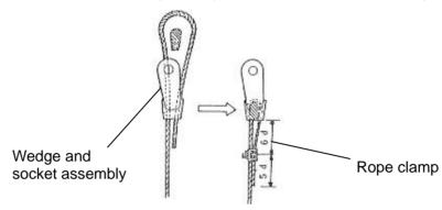
Figure 07 – 14 Socket with Rope Clamp
