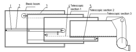
Figure 07 – 15 Telescoping Principle
