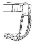
Figure 07 – 8 Down Boom Position
