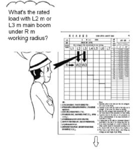
The rated load: If the main boom length is L2 m, the rated load is  $W_2$  kg. If the main boom length is L3 m, the rated load is  $W_3$  kg.
