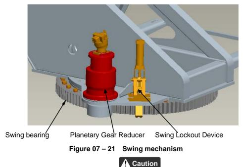
When you turn the crane, your view to the rear and side can be blocked. Be careful. Make sure that work-site personnel and equipment are clear from the area of travel. Send out a short warning sound (horn) before you move the crane. The aft end of the crane extends out 3760 mm from the superstructure center point.
