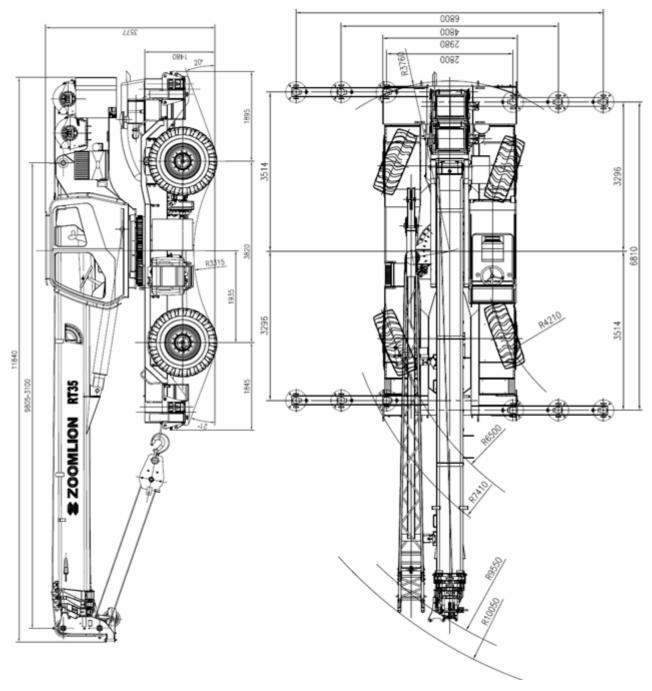
Figure 09 – 1 Overall View – RT35 Rough Terrain Crane
