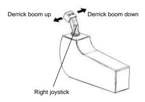
Figure 07 – 27 Derrick + Boom Extend or Retract
