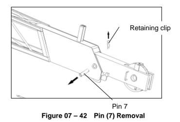
(11) Pull out the section 2, stop when it touches the limit stop. Align the holes and install the pin (7) and the retaining clip.
