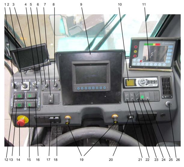
Figure 06 – 1 Upper Controls and Instruments
