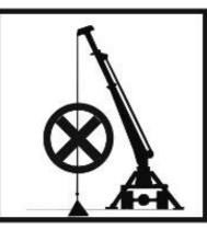
(9) Do not extend / retract the boom with a suspended load.
