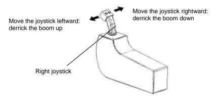
Figure 07 – 19 Derricking Operation
