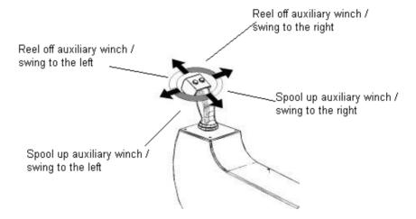
Figure 07 – 32 Swing + Auxiliary Winch
