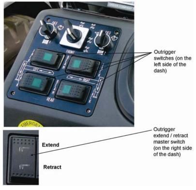
Figure 07 – 1 Outrigger Switches
