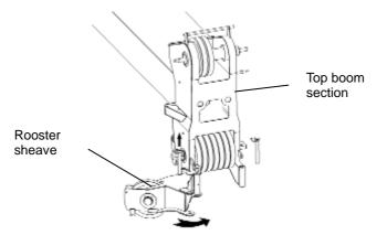
Figure 07 – 50 Rooster Sheave Assembly
