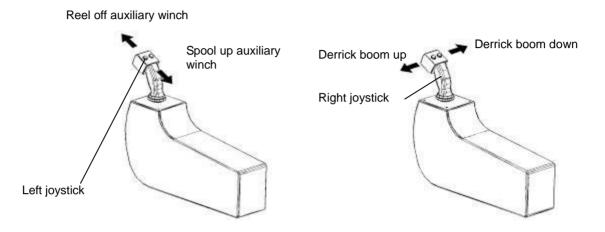
Figure 07 – 28 Derrick + Auxiliary Winch
