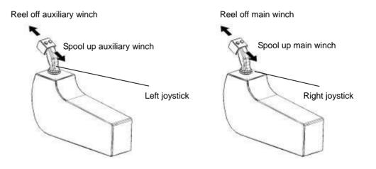
Figure 07 – 26 Main Winch + Auxiliary Winch
