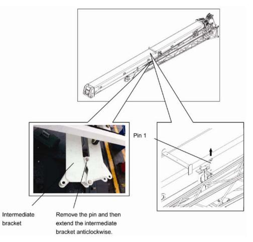
Figure 07 – 36 Pin (1) Removal
