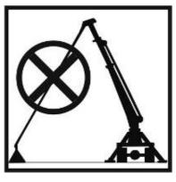
(8) Do not try to lift a load that is buried or frozen on the ground.
