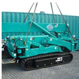
**Four Rigging Points For Lifting Machine**
