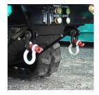
Tie Down Anchors For Transport - Standard on MC Models
