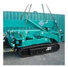
Four Rigging Points For Lifting Machine – Standard on MC305-2 & MC405
