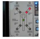
InterLock Outrigger Safety System – Standard on MC Models
