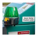
Boom Position Warning Lamp – Standard on MC305-2 & MC405
