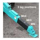
Multiple Position Outriggers (MC305-2 & MC405 shown) - Standard on MC305-2 & MC405
