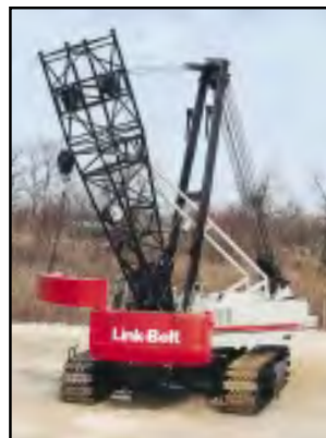
Optional 10' (3.05 m) boom extension handles treadmembers, counterweight and boom during self-stripped down or erection.
