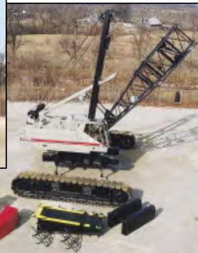
Optional 10' (3.05 m) boom extension handles treadmembers, counterweight and boom during self-stripped down or erection.
