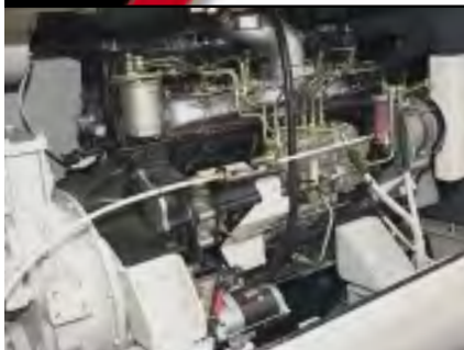
248 hp Isuzu A-6SD1T-QB-01 engine
