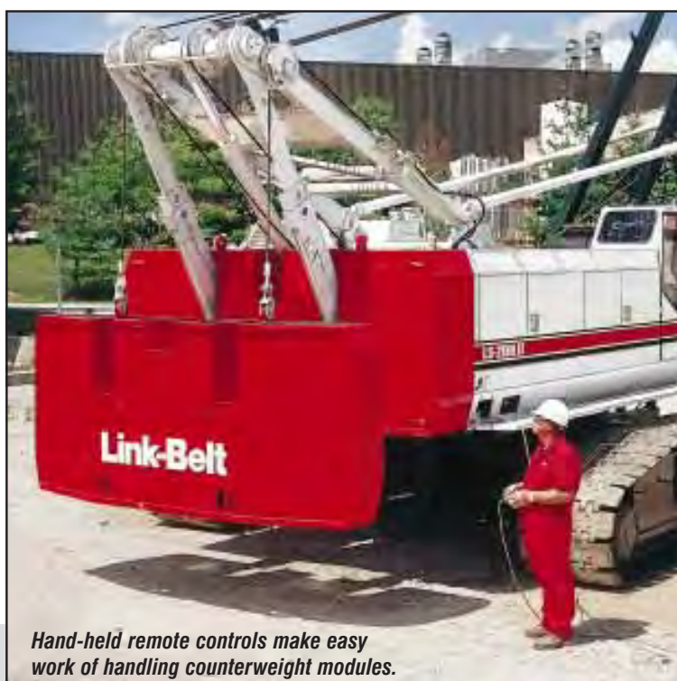
Link-Belt's optional Quick Draw system simplifies assembly, disassembly and counterweight removal
