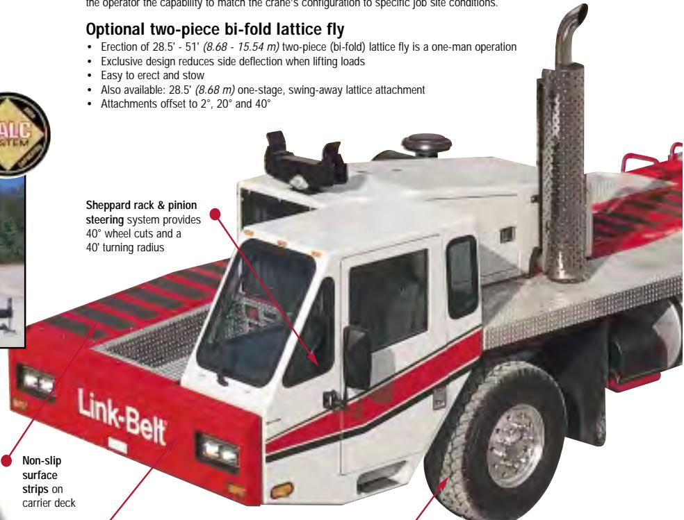
Sheppard rack & pinion steering system provides 40° wheel cuts and a 40' turning radius
