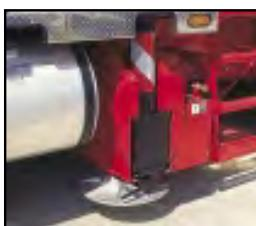
Two standard carrier-mounted outrigger controls, located on each side of the carrier, include a throttle-up switch that brings engine up to 1,200 rpm's for fast outrigger deployment. For fine level adjusting of the carrier, throttle can be taken down to idle.
