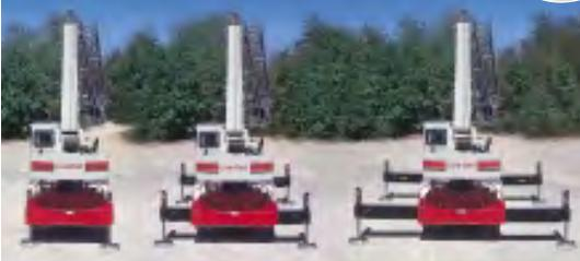
*The Confined Area Lifting Capacities (CALC) system provides three outrigger positions:*
