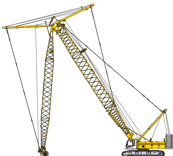
Erecting of main boom and luffing jib
