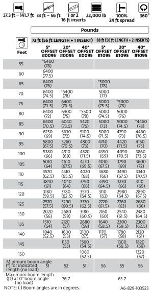
All capacities above the bold line are based on structural strength of boom extension and do not exceed 85% of tipping loads, in accordance with SAE I-765.
