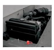
Engine Standard: Cummins QSB 3.3 L turbo-charged diesel rated at 63,4 kW (85 bhp) at 2600 rpm.
