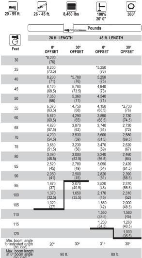
NOTE: () Boom angles are in degrees. \*This capacity based on maximum boom angle. A6-829-101542
