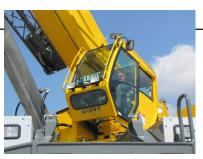
The Full Vision cab on the RT9130E-2 tilts up to 20° providing the operator additional comfort when working at long boom and extension lengths.
