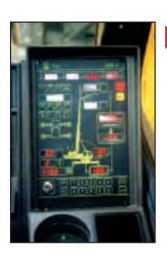
load moment indicator operates in conjunction with ECOS continuously displaying crane configuration and load moment data
