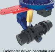
Goldhofer driven pendular axle with ball bearing race ring
