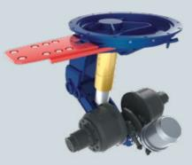
+ Goldhofer pendular axle with ball bearing race ring
