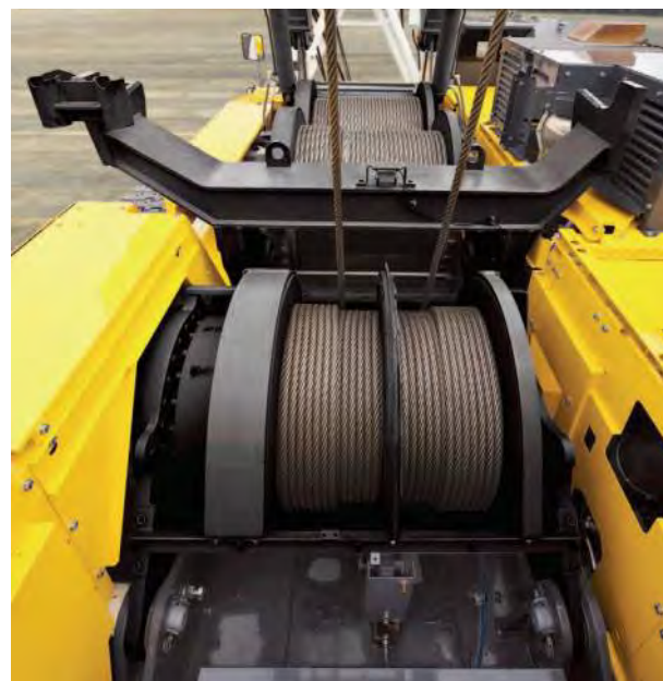
View towards the front of the machine : Front, Rear and Boom drums
