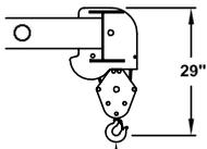
TWO PART LOAD LINE FOR LOADS UP TO 9000 LBS (WT 60 LBS)
